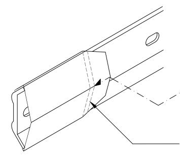
Note: Joints on the fascia bar must be offset by a minimum of 12—inches from the joints in the fascia
